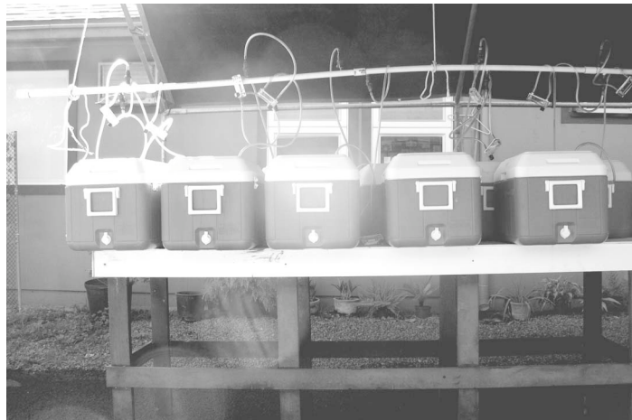
Figure 1. The experimental fingerling transport system (above) used in our study was composed of 24 insulated coolers, each with a 25-L working volume and supplemented with individually metered oxygen supplies.
